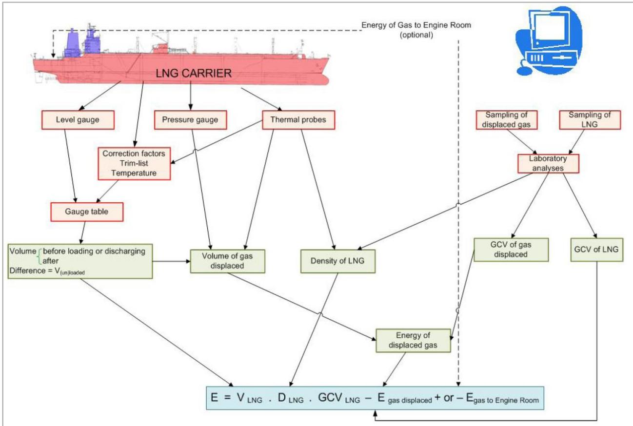
Figure 2 : Determining the transferred energy (using cargo measurement data)
