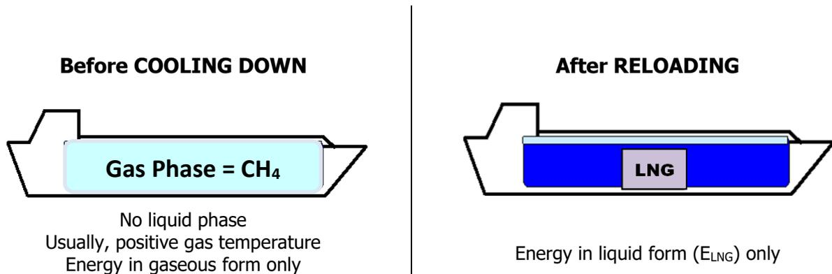
**Figure 4** : Cooling down operation with reloading
